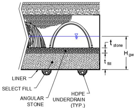
$$H_{gw} \times (62.4 \text{ lb/ft}^3) = [(Y_{stone} \times t) + [(Y_{fill} \times t)] / SF$$
