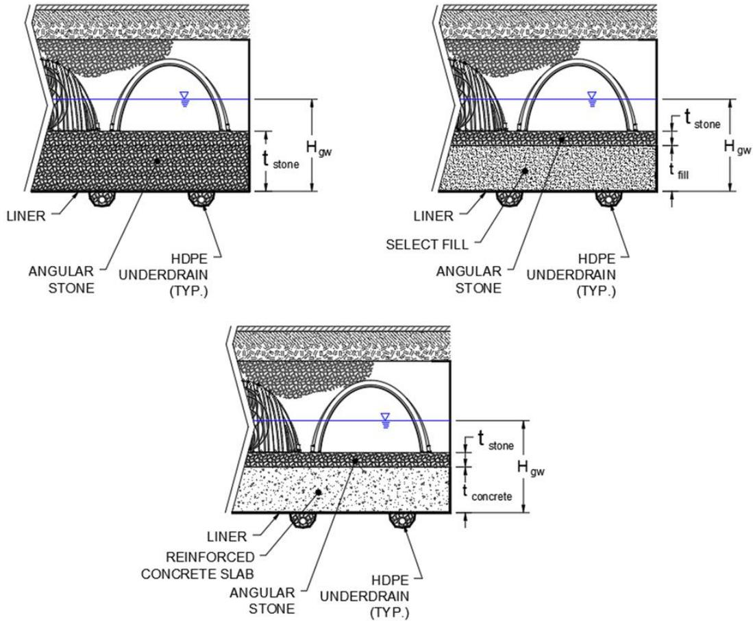
The bedding thickness calculation is simplified by ignoring any structural contribution from the liner and reinforcing material and considering only the weight of the stone or stone/fill in the thinnest area of the bedding, which is located under the chamber.
