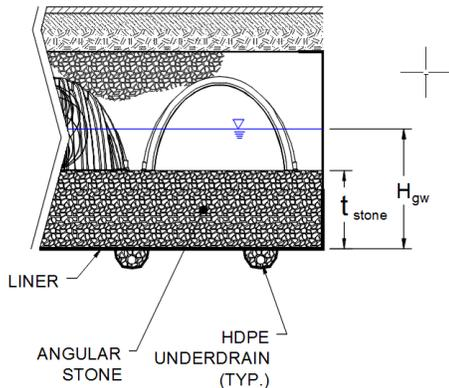
$$H_{gw} \times (62.4 \text{ lb/ft}^3) = [(Y_{\text{stone}} \times t) / SF]$$
